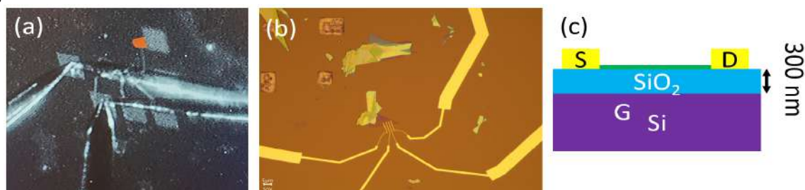
Figure 1. (a) Device as probed in-situ via electrical probes. (b) Microscope image of the 2D flake showing 3 devices contacted by 4 wires. (c) Schematic of a 2D material backgated device. The 300 nm SiO 2 acts as the gate dielectric.
