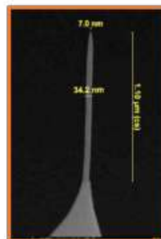
Figure 1. a) W-C FIBID nanoSQUID grown on a flat Si//SiO 2 substrate; b) Fe FEBID tip for magnetic force microscopy.
