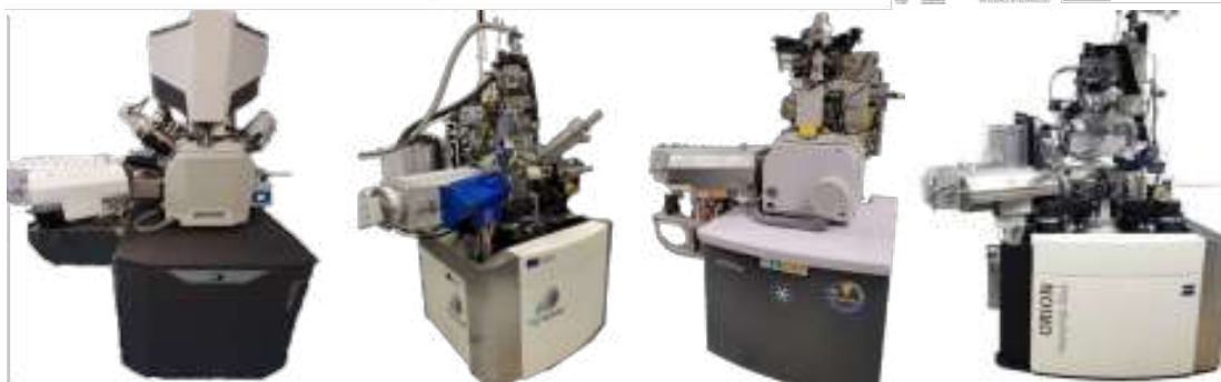
Figure 1. Different FIB platforms equipped with LIST's magnetic sector SIMS system: ZEISS ORION NanoFab Helium Ion Microscope, Thermo Fisher DualBeam, npSCOPE and SIMS:ZERO (left to right).
